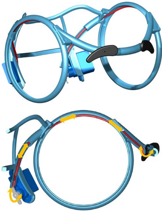
Fig. 2. Actuation of the eyebrows. Top: complete mechanism. Bottom: middle section. The orange arrows show the conversion between rotation and translation.
