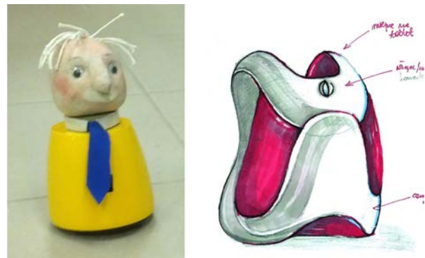
Fig. 2: Different exchangeable casings for universal mobile robot used in therapeutic environment. First: A doll-like shell for a mobile robot. Design by Honorata Lukasik. Second: A soft shell with a place for a tablet for a robotic assistant designed for a therapeutic assistant robot.
